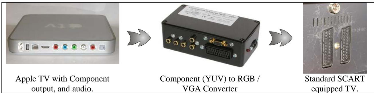
The five phono connectors on Apple TV (the round multi coloured ones) have to be interfaced to the SCART connector on the TV, but we need to convert the type of signal too. That's why we are using a video converter, the **Component (YUV) to RGB / VGA Converter** as shown above.
