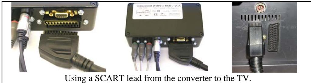
Finally, the SCART can be connected from the converter to the TV.
