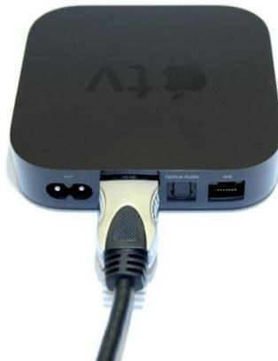
Each option will require that the Apple TV source is connected via the HDMI connection as per the above picture. In some systems the digital audio output and network interface will also be used and more information on these connections can be found on the Apple TV user guide.
