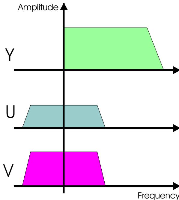
Figure 2. Component video with the brightness (Y) and colour difference signals (U&V).
