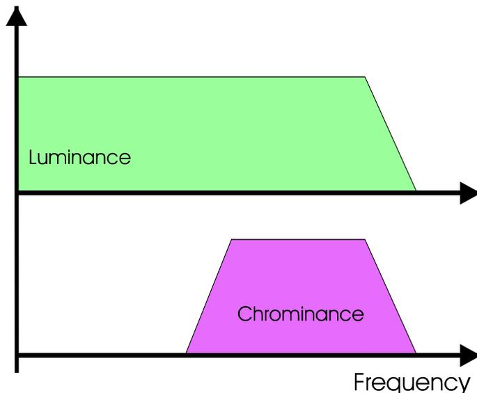
Figure 3a: Frequency Spectrum of S-Video with separated luminance and chrominance.
