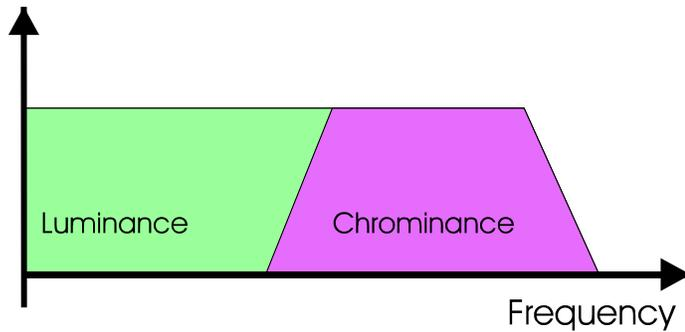
Figure 4a: Frequency spectrum of Composite Video.
