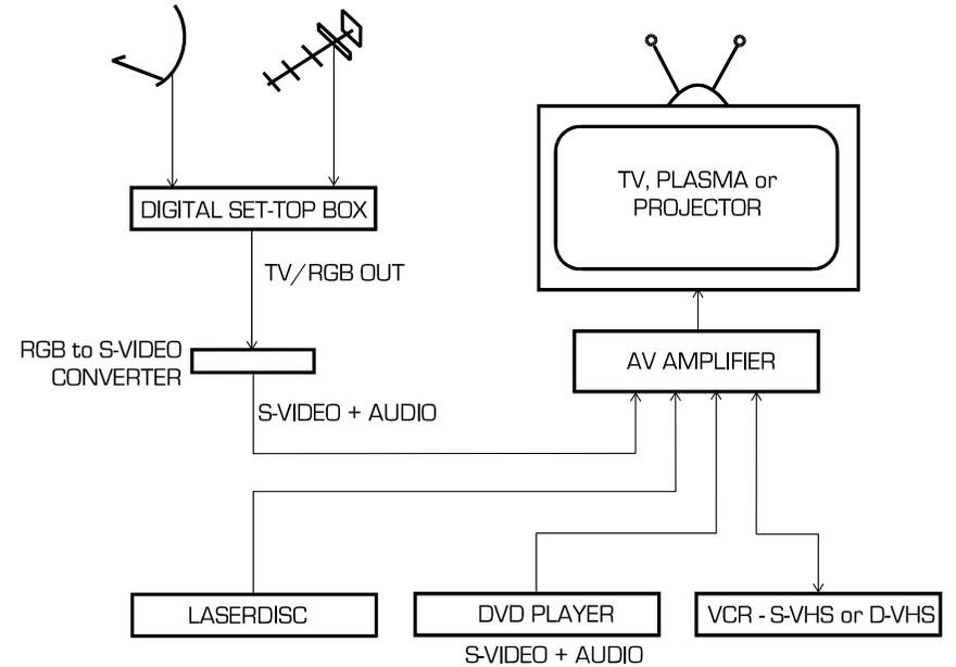
A full configuration is where an AV amplifier acts as a video switch. Several devices are connected to the amplifier, including laserdisc and DVD players. There may be more than one digital set-top box to be connected. Output from the amplifier is connected directly to the TV, plasma or projector. The S-VHS or D-VHS recorder is connected to the amplifier also, although the RGB to S-Video converter could be directly connected to the recorder and the recorder's output connected to the amplifier.
