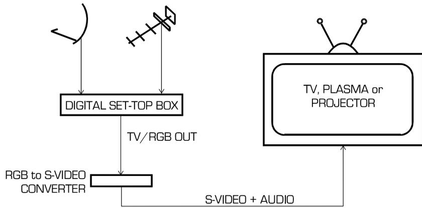
A basic configuration is to connect the digital set-top box (or DVD player) to the converter's SCART input, then the output directly to the TV, plasma or projector.
