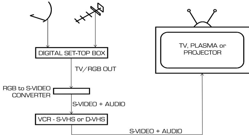
If the home-cinema system has a S-VHS or D-VHS recorder, then it would be appropriate to connect the RGB to S-Video converter to the TV, plasma or projector via the recorder.
